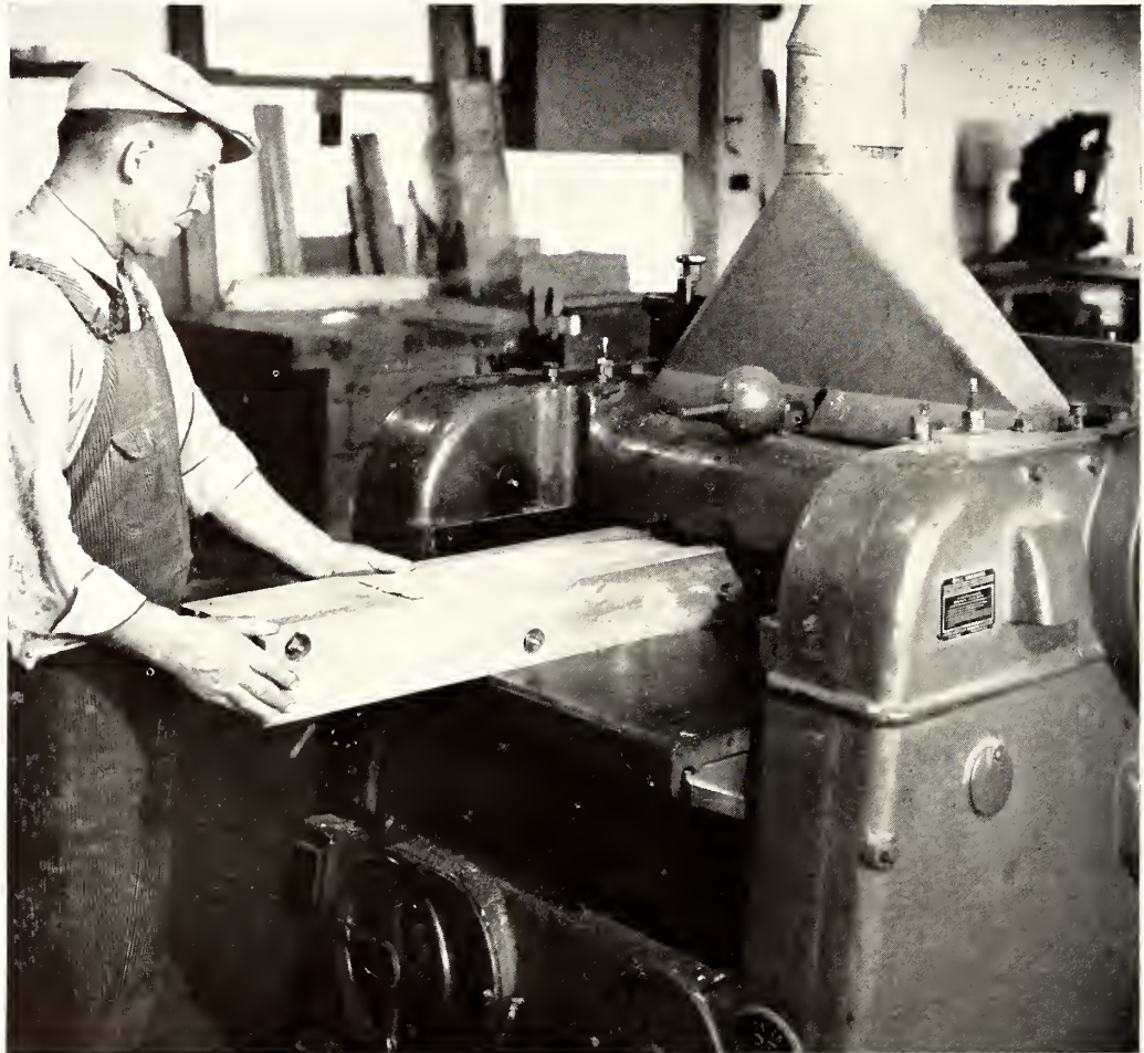
FIGURE 5-67.—Cutting a scarf joint on an ordinary single-head cabinet planer.
